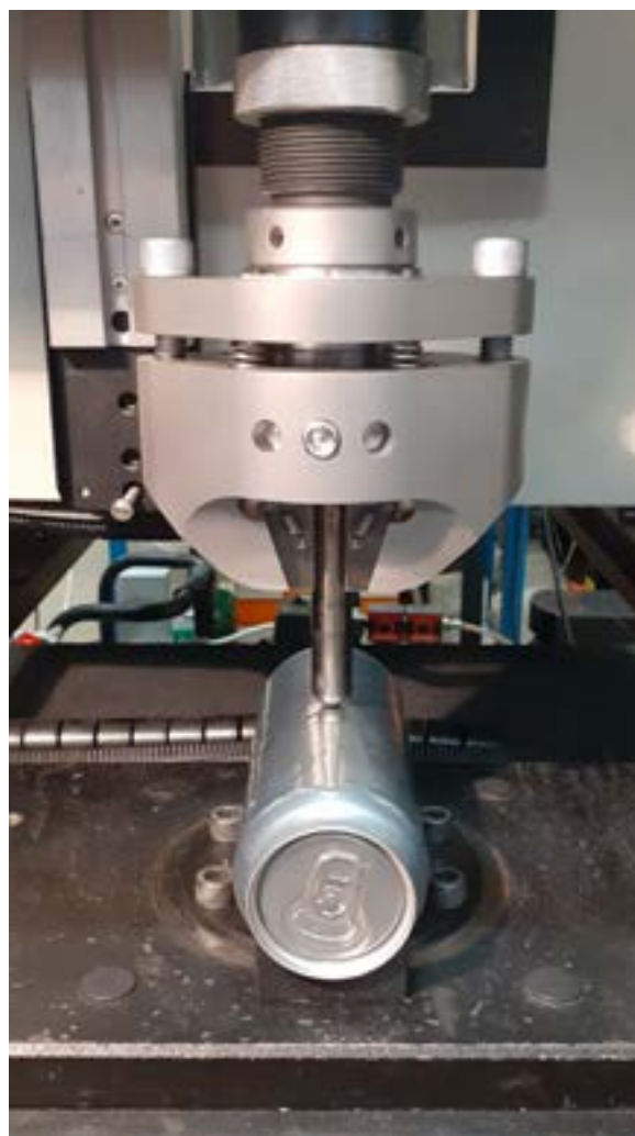
Figure 1 Instron apparatus with sample can
