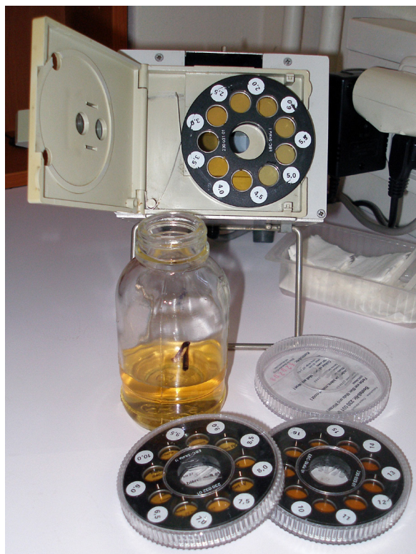
Figure 2 The comparator for determination of malt colour
