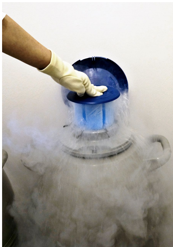
Figure 1 Cryopreservation of the brewer's yeasts in the cryogenic Dewar vessel filled with liquid nitrogen in RIBM laboratory
