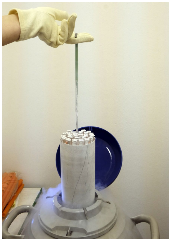
Figure 2 Pulling up of test tubes with brewer's yeasts from the cryogenic Dewar vessel filled with liquid nitrogen
