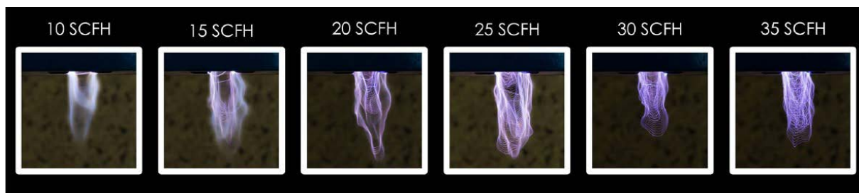
Figure 2 The transition between flame to filamentary mode of Gliding Arc discharge
