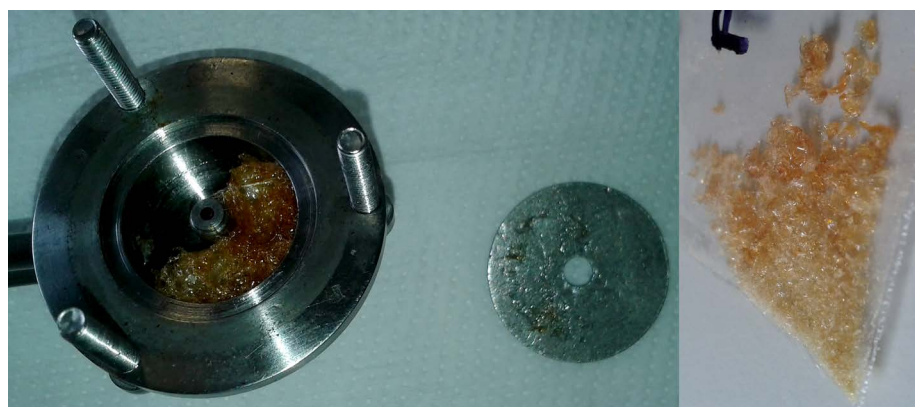
Figure 7 The crystallized resin-like matter on the permeate side of the membrane
